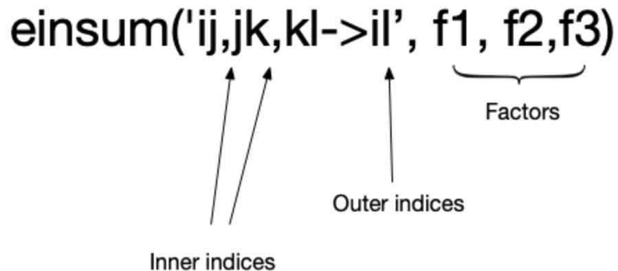
The diagram shows the notation `einsum('ij,jk,kl->il', f1, f2, f3)`. Below the opening quote, two parallel arrows point upwards to the indices `ij` and `jk`, with the label "Inner indices" centered below them. A single arrow points upwards from the label "Outer indices" to the index `il` after the arrow in the quote. A horizontal curly brace is positioned below the closing quote and the factors `f1, f2, f3`, with the label "Factors" centered below the brace.
